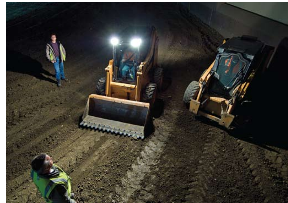
Standard lights on the 445 cast beams straight ahead (top), leaving objects to the sides in shadow (note the dome-lit 445 Series 3 to the right, and there is a reporter lurking to the left). When the machines change places, the Series-3 standard side lighting clearly shows hazards in the loader’s skid-steering space.
